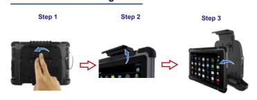
1.Slide the latch to open the hook
