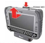
1. While holding the M9020, press the release latch on the docking station and then lift the device to un-dock it.
