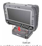
1. Align the golden connector and guide pin holes on the M9020 with one on the docking station. Insert M9020 into the guide pin holes on the docking station
