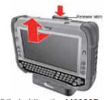
1. While holding the M9020B, press the release latch on the docking station and then lift the device to un-dock it.
