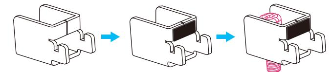
• Step 3. Hook the mounting clamp into the corresponding mounting pair slots of the display. Then fasten the clamp with the included mounting screw to secure its position on the sub frame or panel. Repeat the same procedure for the remaining mounting clamps
