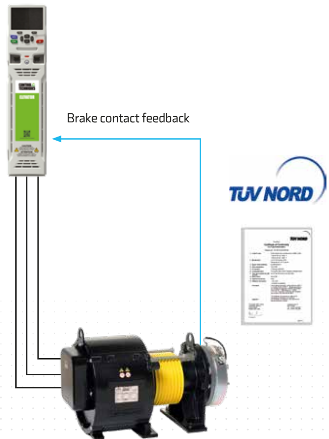
TÜV certified Brake Contact Monitoring functions on the elevator drive E300
