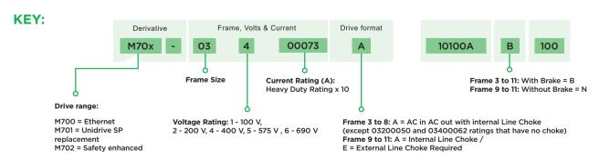
For configurations involving frame size 9 and above refer to the Unidrive M: High Power Modular AC Drives brochure
