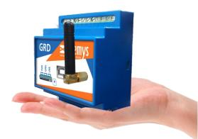
The GRD family of products helps control and supervise any kind of equipment from distance, be it a control system or process system facilitating the implementation of the remote telemetry systems. Additionally it includes the possibility to load a text script to perform internal logics.
