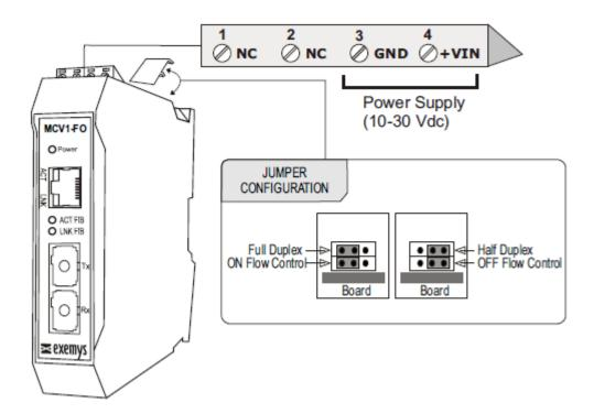
There are two configuration jumper switches, both to configure the converter's operation, from the optic fiber side:
