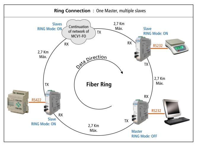
To use the ring mode each of the MCV1-FO that connected to the slaves must have the Jumper of Configuration in RING MODE in ON position, also the Master must have the RING MODE in OFF position.
