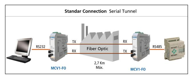
The use of the MCV1-FO also allows you convert the type of serial (RS232, RS485 or RS422), that mean that you can connect to the equipment two different type of serial in each one of the ends of the tunnel.
