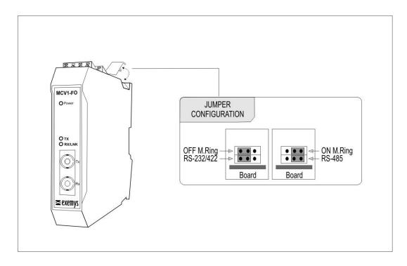
There are two configuration jumpers. They will determine how the converter will work.
