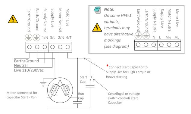
Extra starting torque may be needed for loads which have a particularly 'sticky' starting characteristic. This can be achieved by rearranging the internal connection of the starting capacitor, bringing the connection out and to the supply side of the starter as shown.
