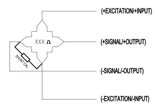
FOR POSITIVE OUTPUT DURING SHUNT CALIBRATION, RESISTOR MUST BE CONNECTED ACROSS -EXCITATION AND -SIGNAL
