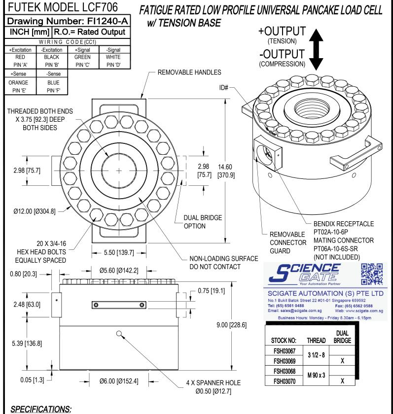
RATED OUTPUT CAPACITY SAFE OVERLOAD ZERO BALANCE EXCITATION (VDC OR VAC) **BRIDGE RESISTANCE NONLINEARITY HYSTERESIS NONREPEATABILITY**
