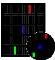
Cluster pixel defect type 3a Sub-pixels in a cluster area constantly lit
