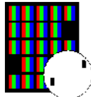
Cluster pixel defect type 2 Pixels in a cluster area constantly dark
