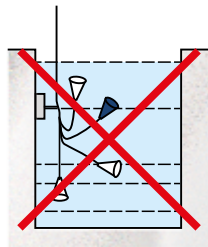
Image 6. Avoid fixing the float such that a sharp corner can cause kinks or wear to the cable.
