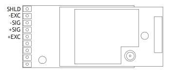
The resistance of the strain gauge can be between 85 and 5000 Ohms. The T24-SA can support up to 4 3500hm strain gauges bridges attached in parallel (At the expense of reduced battery life).
