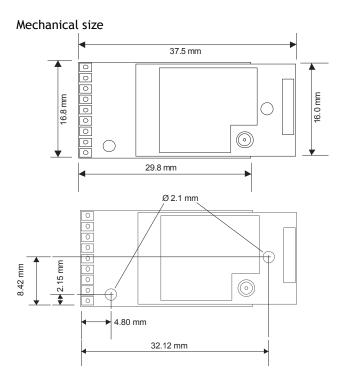
There are two holes available for mounting. The one nearest the connection pads can accept an M2 screw or American equivalent #0-80. Important Note: DO NOT USE #2 screw size. Note that the mounting hole is connected directly to the Battery ground of the acquisition module. The mounting hole near the chip antenna cannot accept metal mounting hardware.
