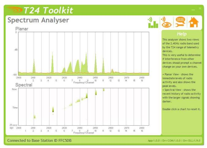
The analyser page is provided as a tool and will not normally be needed unless you plan to change channels and want to find the best channel to select, or to diagnose poor communications issues.
