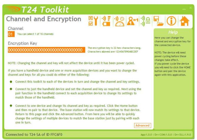
Here you can change the channel and encryption key for the acquisition module device. If you want to change the channel of an acquisition module and T24-HS pair there is no need to change both devices.
