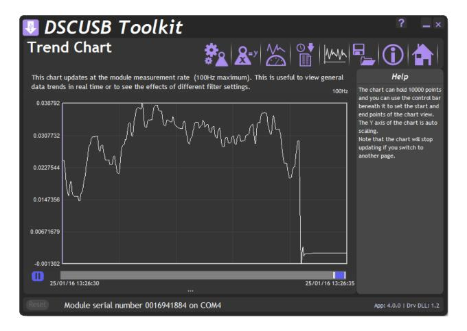
Data will be read from the module at the **Measurement Rate** (up to a maximum rate of 100Hz) and added to the trend chart. You can see the current rate at which data is added at the top right of the chart.
