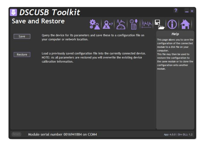
Clicking the 'Save' buttons will allow you to specify a file to which the configuration of the connected module is written.
