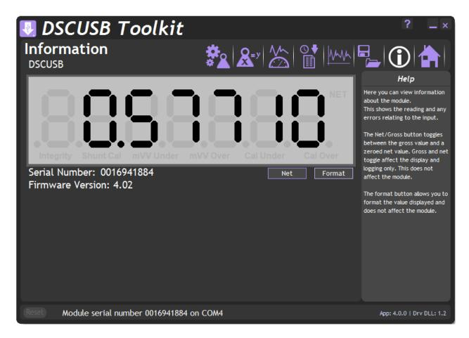
This simply shows a large display and indicates if any error conditions are present by displaying an information box. If the module has been allocated engineering units these may be displayed in the upper right of the LCD display.
