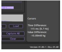
This displays the time difference between the two cursors (Plus the frequency if you had placed the cursors on two adjacent features in a wave based signal) and the value difference.
