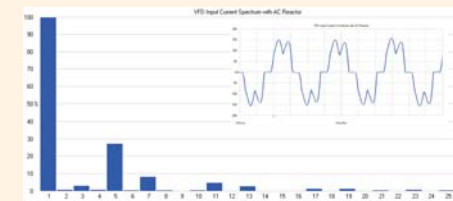
VSD Input Current Waveform and Spectrum with AC reactor.
