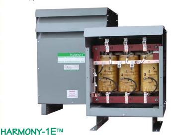
Superior to K-rated and conventional transformers in reducing voltage distortion (flat-topping) and power losses due to current harmonics created by single-phase, non-linear loads such as computer equipment. Secondary windings arranged to cancel zero sequence fluxes and eliminate primary winding circulating currents. Treats triplen harmonics (3rd, 9th and 15th) within the secondary windings and 5th and 7th harmonics upstream.
