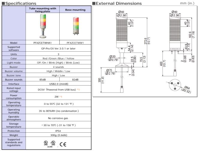
\*1 In case to connect with GP4000M, need external power supply for USB port.
