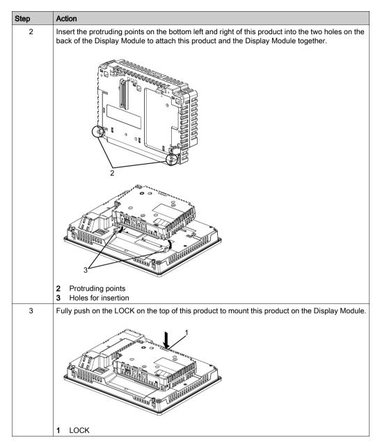
**NOTE:** Refer to the SP5000 Series Hardware Manual or the SP5000 Series (Display Module) Installation Guide on how to mount the Display Module to the panel.
