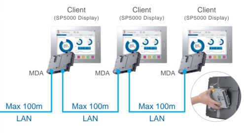
Distance: 100M between host and external monitor Wiring: 1 LAN cable for both video & touch signal
