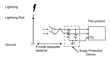
• Attach a surge protection device to prevent damage to this product as a result of a lightninginduced power surge from a large electromagnetic field generated from a direct lightning strike. We also strongly recommend to connect the crossover grounding wire of this product to a position close to the ground terminal of the surge protection device.
