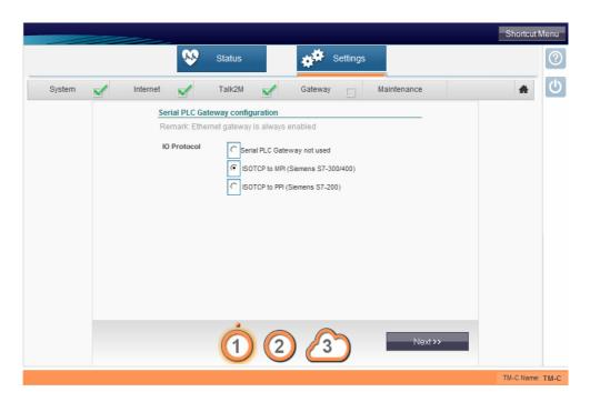
Select the suitable IO protocol. In this case ISOTCP to MPI (Siemens S7-300/400) and click [Next>>].
