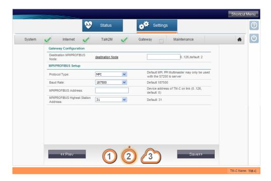
Enter the communication settings of your PLC and select the used protocol. After that click [Save>>] to finish and to activate the gateway configuration.
