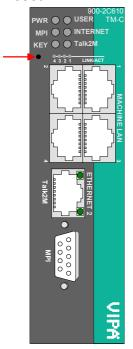
A reset at the Teleservice module may be initiated by the Reset button The Reset button is allocated below the LEDs behind an opening. Please use for operation a pointed object.
