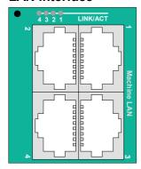
You may connect your TM via Ethernet to the local machine network. Via Ethernet the integrated Web page of the TM module may be accessed for according configurations.
