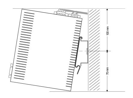
Insert the module that you are installing into the profile rail at an angle of about 45 degrees from the top and rotate the module into place until it clicks into the profile rail with an audible click.
