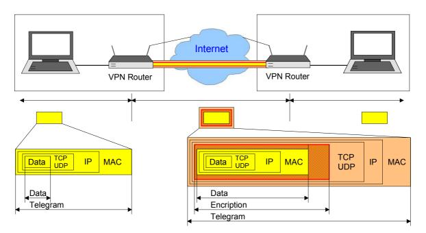
Talk2MTalk2M (Talk to Machine) is a service, by means of which you may reach<br/>your plant word-wide via cellular radio or DSL/LAN. Talk2M communicates<br/>fully secured over VPN. Since Talk2M only uses outgoing connections,<br/>problematic points like firewalls, missing open ports and dynamic IP<br/>addresses may be handled
