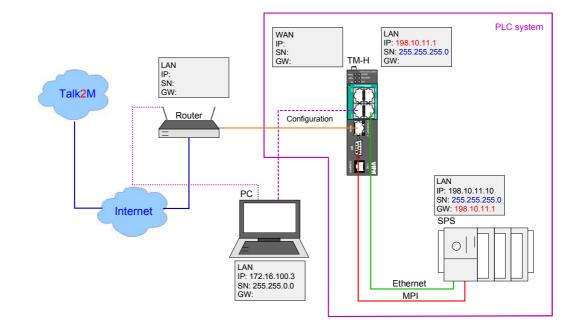
Connect TM to Talk2M via DSL/LAN Start the program eCatcher. If the connection to the Talk2M server was successfully established, the configuration dialog is shown. The configuration dialog is divided into 2 parts.
