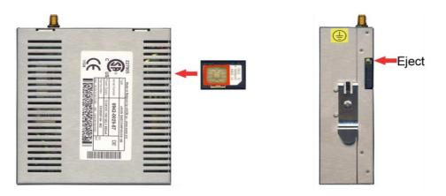
• For taking the SIM cart push the eject button with a pointed object. The eject button may be found above the card slot.
